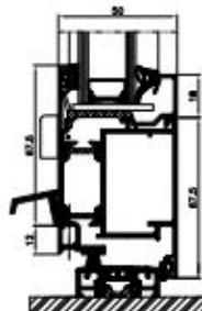
Cross-section of the bottom rail in door
